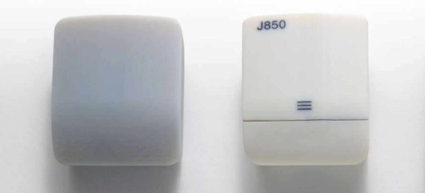
Earbud case prototypes 3D printed with DraftGrey (left) and VeroPureWhite (right)
