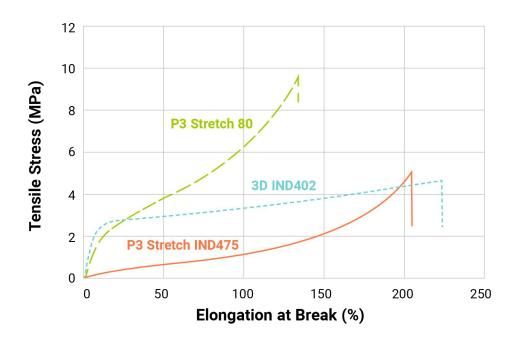
A stress-strain curve of Loctite 3D IND402 and P3 Stretch IND475 show their difference in physical behavior. Loctite 3D IND402 shows high initial resistance to stretching meaning it is more resilient and has more "springiness." P3 Stretch IND475 shows low resistance until breakage indicating it is a softer-touch material.
