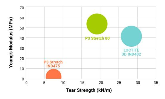
Higher Young's Modulus values indicate that the material is stiffer and has a higher Shore Hardness value. Elastomers with higher stiffness are generally more resistant to tearing.
