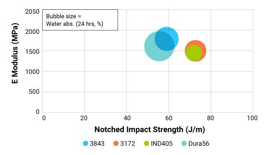
Origin has a robust portfolio of tough materials featuring different colors, performance profiles, and cost points. The three materials shown above are good choices for parts and applications in high impact environments (manufacturing jigs) or frequently opened and closed (latches).
