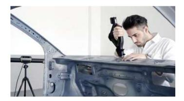
It can be paired with a portable prober (optional with different sizes) to probe inaccessible areas such as holes and hidden points. This contact measurement probe can ensure precise results with high single-point repeatability of 0.030 mm.
